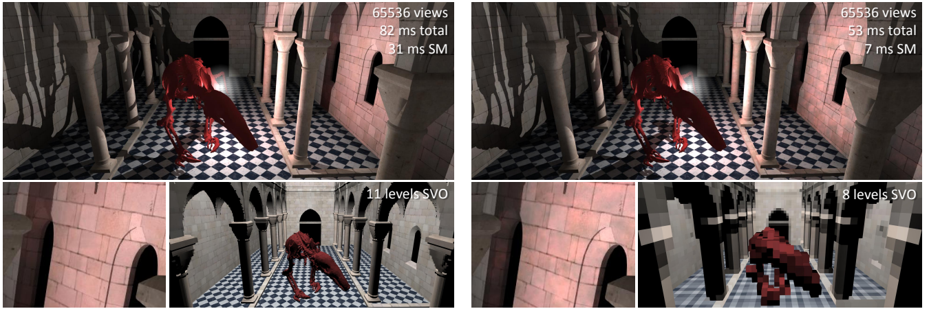
Figure 13: Effect of hierarchy resolution in the Sibenik scene. While the shadow map rendering cost is significantly reduced, using a too low hierarchy resolution causes inaccurate shadow maps, resulting in missed or exaggerated occlusions and artifacts.
