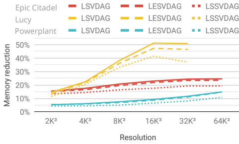
Fig. 11. Memory reduction comparison of the LSV DAG relative to the SVDAG, the LESV DAG relative to the ESVDAG and LSSV DAG relative to the SSV DAG.
