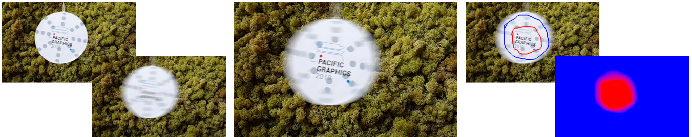
Figure 1: Left: single frame from 240Hz short-exposure video and a simulated long exposure at 30Hz by averaging 8 frames. Middle: Using the 240Hz input, our method enables mixing a long exposure in the periphery with a short exposure for the details on the pendulum. Via user annotations in the video, different shutter functions can be defined (top right). Annotations and shutter functions can be keyframed over time. Based on the annotations, our method defines an interpolated shutter function for each pixel (bottom right).
