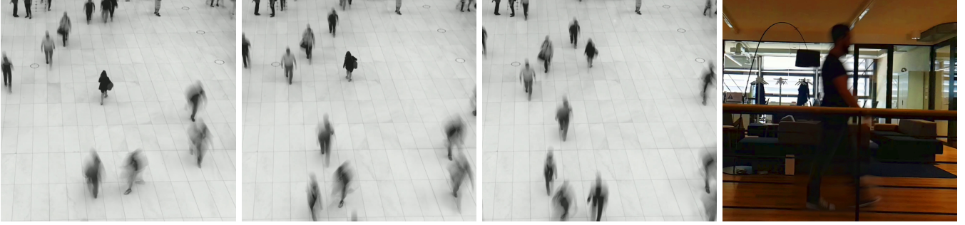
Figure 10: A motion blur shutter can be applied selectively to different regions of the image. Here, the keyframed regions track a person in the images. In the left images, we keep one moving person sharp over a short time span, while blurring the rest. This highlights and draws attention to the person. On the right, we do the opposite, and remove attention from the person crossing the hall. Left video source: pixabay.com at 25Hz. Rendering time (avg): 1.93ms in 960×540. Right image sequence captured in house at 240Hz. Rendering time (avg): 1.58ms in 1280×720.
