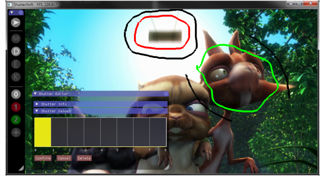
Figure 5: Interface for interactively defining shutter functions and their influence regions. Users design shutter functions using the bar graph editor, whilst additional details, such as the number of frames in the function, can be changed using one of the collapsed fold-outs. Influence regions are defined by drawing scribbles using the corresponding color. The results are immediately visible. The sequence is from the Big Buck Bunny movie by the Blender Institute [Goe08].
