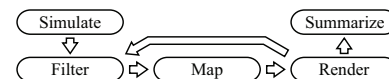
Figure 2: The analysis cycle as described by Upson et al. in [12]. Simulation data is filtered, mapped, rendered, and studied yielding insight, which can be used to initiate a new round of filtering.
