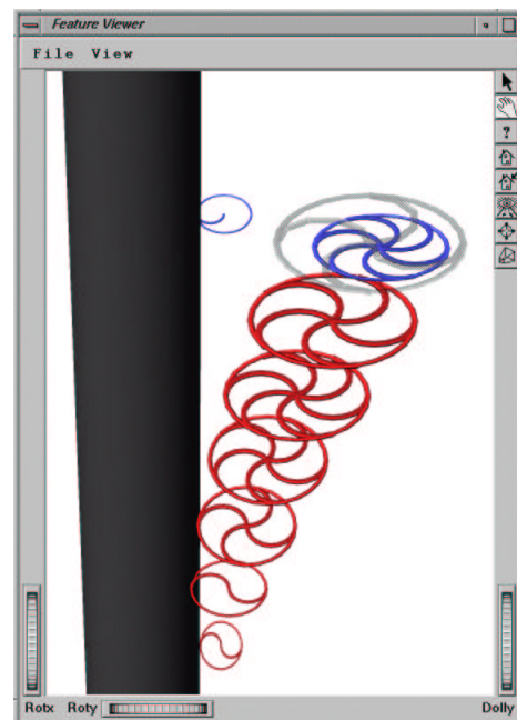
Figure 5: Tracking 2D vortices in space ( z -direction) in order to obtain 3D vortices at one instance of time.
