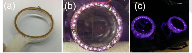
Figure 4: Eye illuminating lens holder. 3d printed lens holder with manufactured circuit board (a), working infrared SMD-LED array (b), illumination units within the HMD (c).
