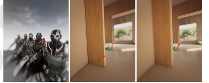
Figure 9: Real-time Gaze-contingent Rendering. Foveated rendering (left): Rendering quality and saturation is decreased for peripheral vision. Adaptive depth-of-field effect (center, right): near and far focus distances. Gaze vector shown as red marker.
