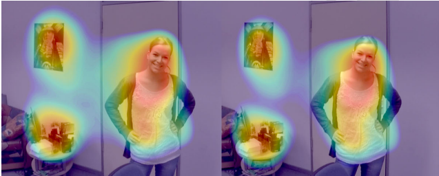
Figure 11: Gaze visualization. Gaze maps for images or videos show the fixated display area averaged over time or users. Temperature color scheme represents fixation quantity.
