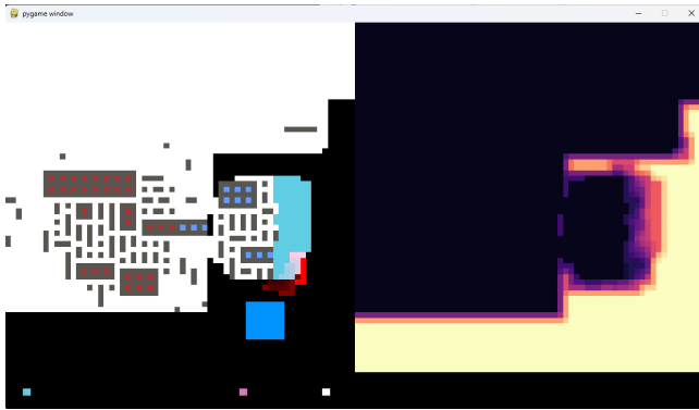
Figure 4: A screenshot of the current pygame-based prototype editor while collapsing meta-tiles into leaf-tiles, combining the overlapping model with hierarchical semantic WFC.
