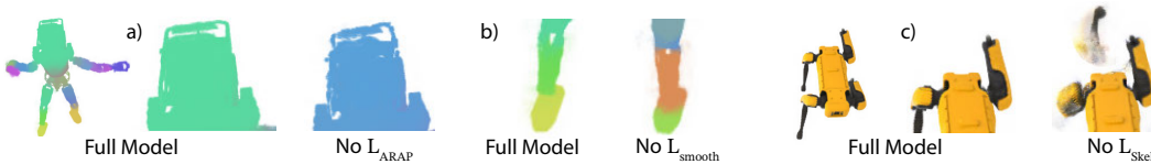
Figure 9: Ablation examples. a) \mathcal{L}_{ARAP} enforces rigidity after pruning (see upper pipes), b) \mathcal{L}_{smooth} results in better part-segmentation, c) \mathcal{L}_{skel} enforces the joints to stay inside the shape.
