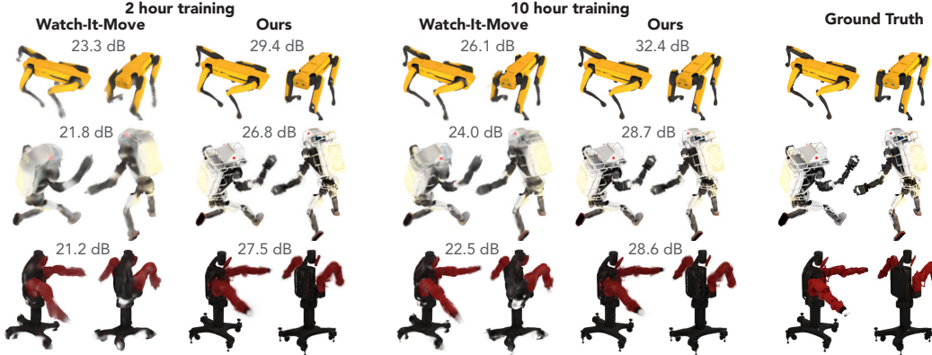
Figure 3: Qualitative comparison displaying two held-out views-frames of scenes from the Robots rendered by WIM [20] and our method after 2 and 10 hours of training, and the PSNR scores.
